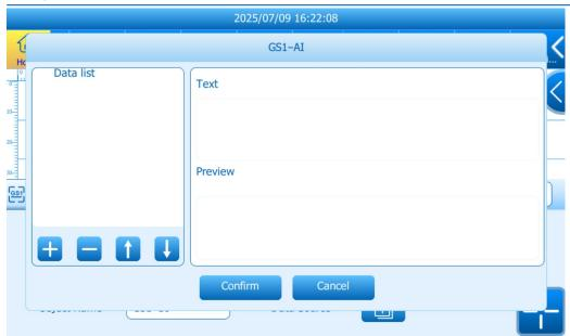
Tap to open the GS1 Al code checklist. You can select individual GS1 Application Identifiers (Als) and enter their corresponding data based on the their encoding rules.
