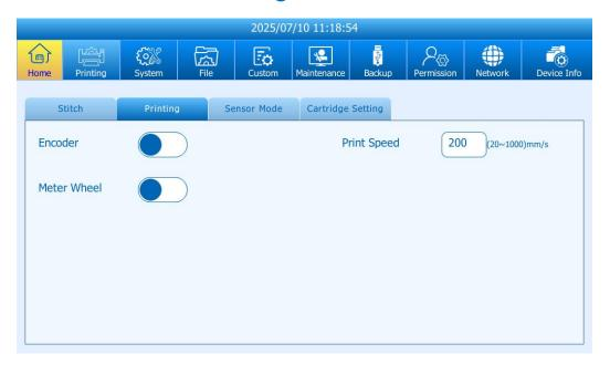
**Encoder:** Enable or disable the external encoder. By default, it is off. When enabled, the encoder automatically detects print direction and speed. When disabled, you can manually set the print speed to match the conveyor speed (20–1000 mm/s).
