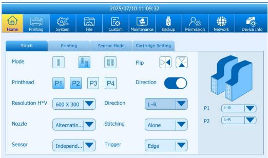
**Resolution H\*V:** Set the horizontal and vertical print resolution. The default is 600 DPI (horizontal) × 300 DPI (vertical).
