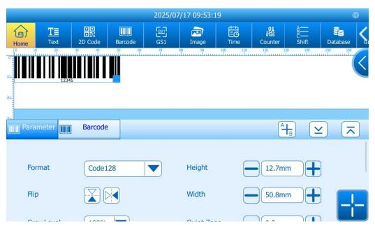
**Encoding**: The default format is Code 128. To choose a different option, scroll down and select from the drop-down menu.
