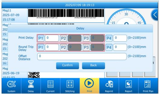
**Round trip Print**: Enable this function to alternate the printhead's movement between forward and reverse directions. It prints once in the set direction, then once in the opposite direction, repeating the cycle.
