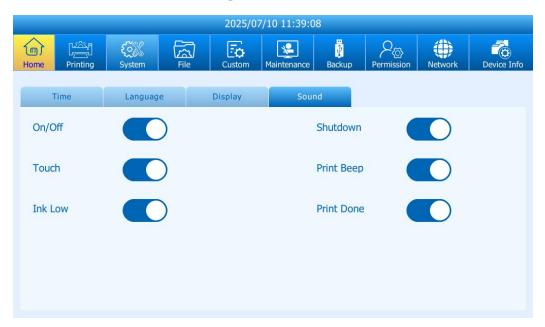
You can enable or disable sound alerts for the printer—such as shutdown tone, touch feedback, print start beep, low ink warning, and print completion beep—by toggling each option on or off in this sound alarm settings menu.
