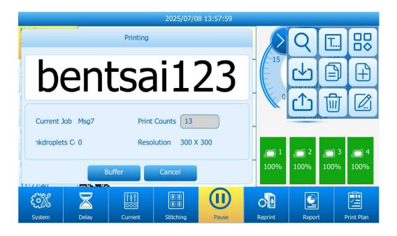
During printing, the displayed message updates in real time to match the actual output. At the same time, the bottom function bar remains active, giving access to **System, Delay, Print Report,** and **Print Plan**—but these options are only available when the print message includes counter or database elements.
