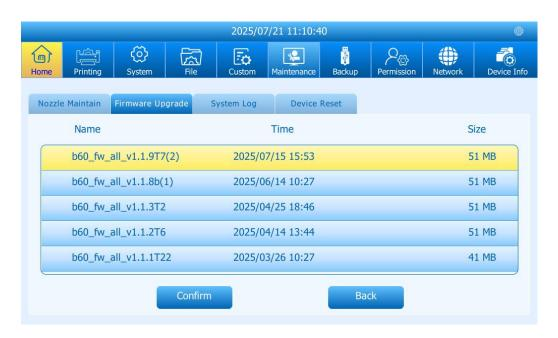
If multiple files are included, install them one by one. Once the upgrade is complete, the printer will shut down automatically.
