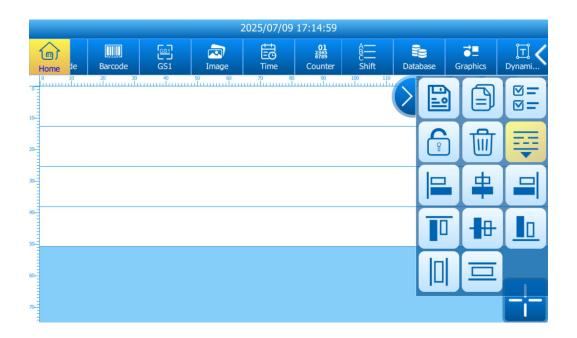
Tap the button to display the object adjustment functions. tap again to hide the right-side menu list.
