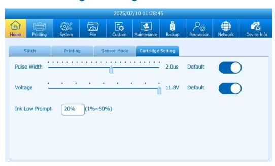
**Pulse Width & Voltage:** When using Bentsai cartridges, default settings are automatically applied based on the cartridge's chip data. For third-party cartridges or custom adjustments,
