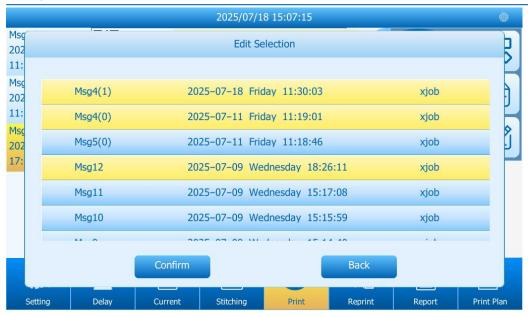
Select messages to include in your print plan and specify the **print count** (Times) for each message. You can also set the **Loop Count** to define how many times the print plan should repeat the sequence.
