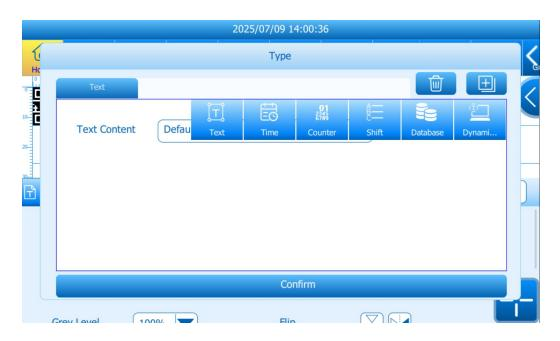
Add: Tap the button to enter the objects adding interface. You can choose from the following types: Text, GS1, Date, Counter, Shift, Database, or Dynamic Text. After selecting a type, you'll be taken to its corresponding editing interface.
