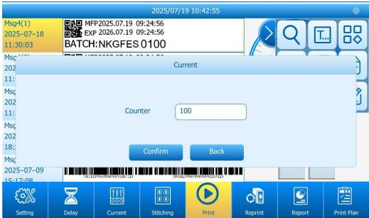
**Note**: This function is available only when the print message includes counter or database objects. Without these elements, the feature will remain inactive.
