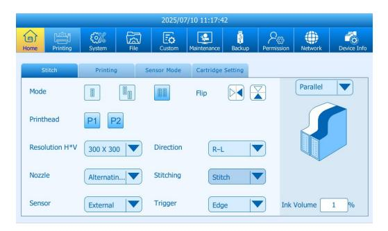
**Alternating:** Alternating printing allows two printheads to work alternately. You can set Printhead 1 to switch to Printhead 2 after reaching a specified usage percentage.
