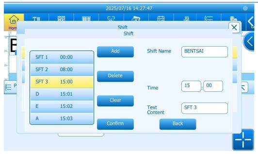
**Add:** Tap **Add**, then enter the shift name and its start time. Next, input the message in Text Content to be printed, and tap **Confirm** to save it to the shift list.
