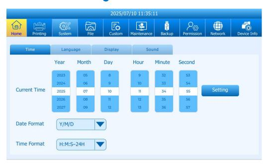
**Current Time:** Set or adjust the system time displayed on the printer by sliding up or down.
