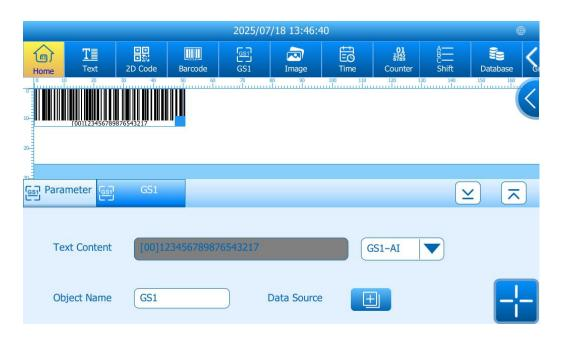
**GS1-AI:** Tap to enter the GS1 AI editing interface. AI fields must be added sequentially to generate a GS1 code. Each AI must follow GS1 code formatting rules.
