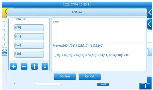
**Object Manager:** GS1 objects can be associated with: text, date, counter, shift, database, dynamic text. For specific operations, refer to the **Object Manager in 5.3.2.**
