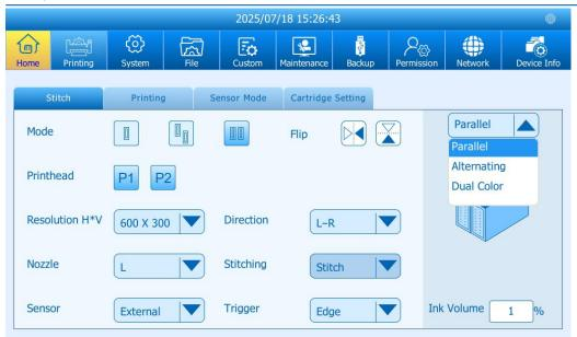
**Parallel:** Parallel mode ensures continuous printing during cartridge replacement. You set ink usage limits for each cartridge. When P1 reaches its limit, the system automatically switches to P2. While P2 is active, you can replace P1 without halting production. Once P2 hits its target, printing switches back to P1—keeping operations uninterrupted.
