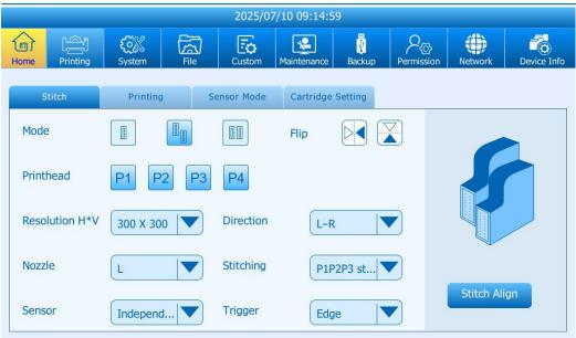
In Stitch Mode, printheads can be selected as needed and used for printing according to the existing stitch mode. Stitch parameters can also be adjusted on this interface. For instructions on stitching alignment, please refer to **Section 6.3.**
