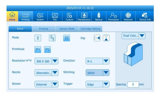
**Flip:** Configure the printhead's image orientation. Options include horizontal and vertical flip to adjust printing direction as needed.
