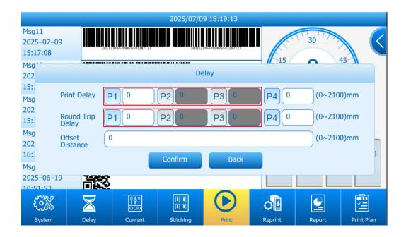
Independent Delay: Allows setting individual delay distances for each selected printhead.
