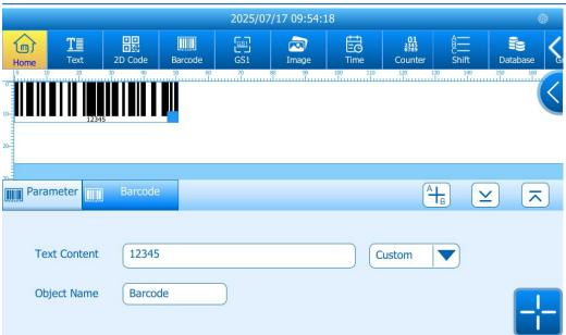
**Text content:** After selecting the barcode format, enter the corresponding text here. Please follow the encoding rules of the selected barcode type—invalid input will trigger an error. If Code 128 or GS1-EAN128 is selected, you may use date or counter as the encoding content.
